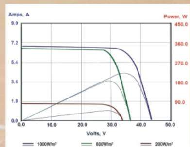
Standard test conditions (STC) 1000W/m<sup>2</sup>, AM 1.5, 25 °C
